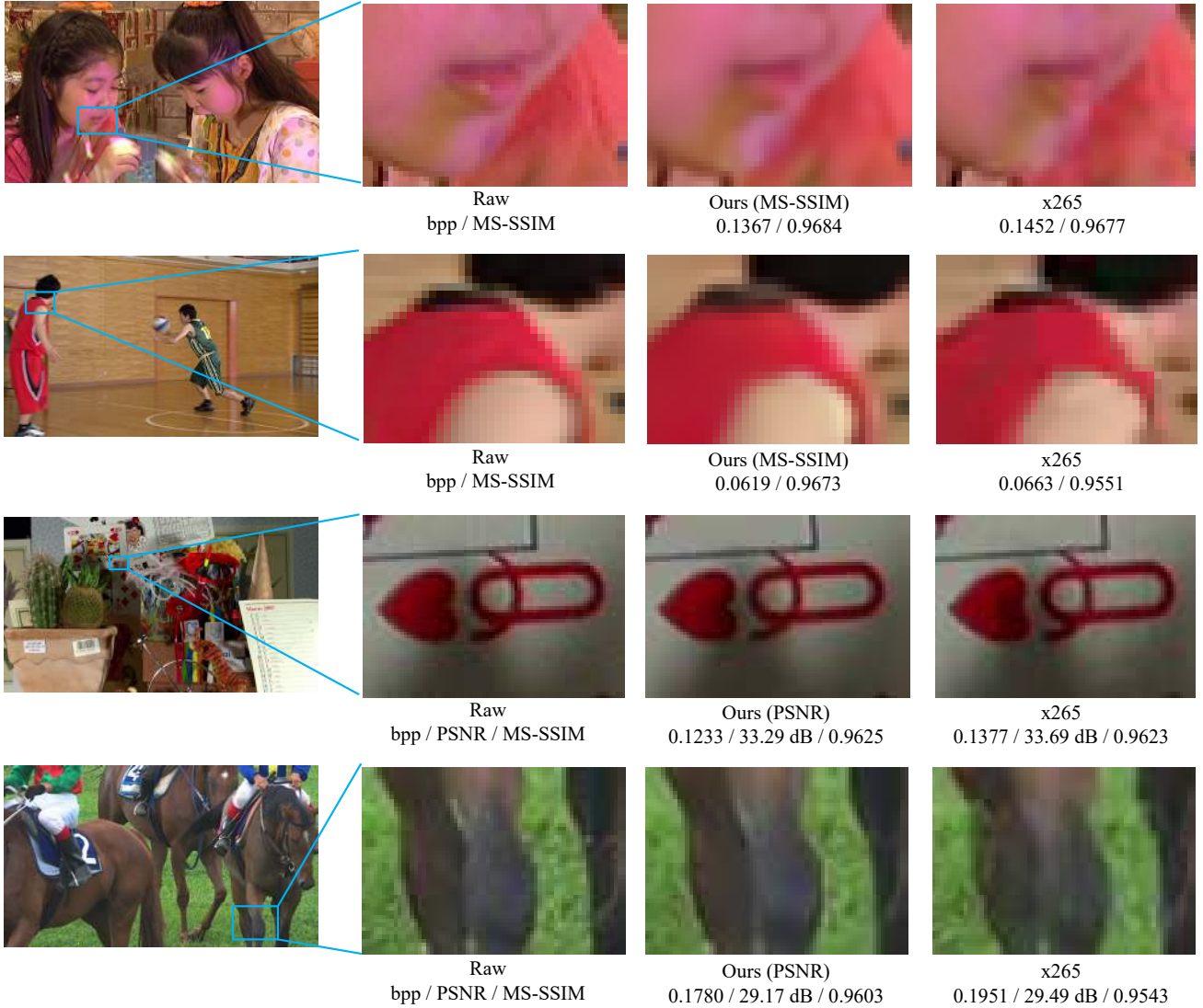
Fig. 8. The visual results of the MS-SSIM and PSNR models of the proposed RLVC approach in comparison with the default setting of x265.
