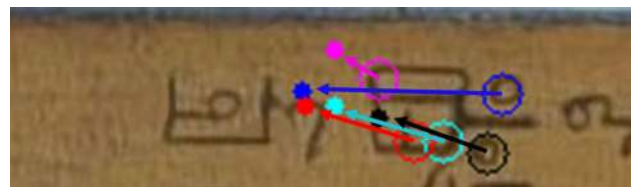
Fig. 5 This figure shows five detected features in part of a test image and the corresponding centre of an expected pattern. This pattern is part of an image from the École française d'Extrême Orient [EFEO], Pondicherry branch
