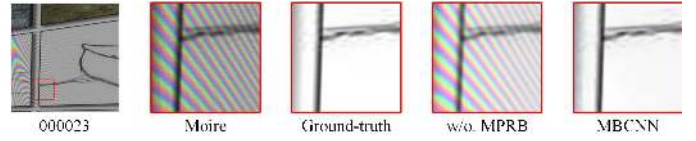
Fig. 8. Demoireing results produced by MBCNN with and without MPRB.
