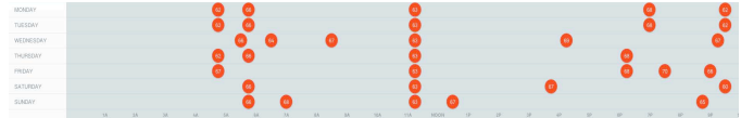
Figure 2. P9's Nest schedule showed frequent temperature changes on certain days. Time is plotted on the X-axis and weekdays are plotted on the Y-axis. The dots show the temperature setting at the particular day and time.
