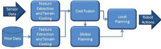
Figure 11: A high level block diagram of the Crusher Autonomy system
