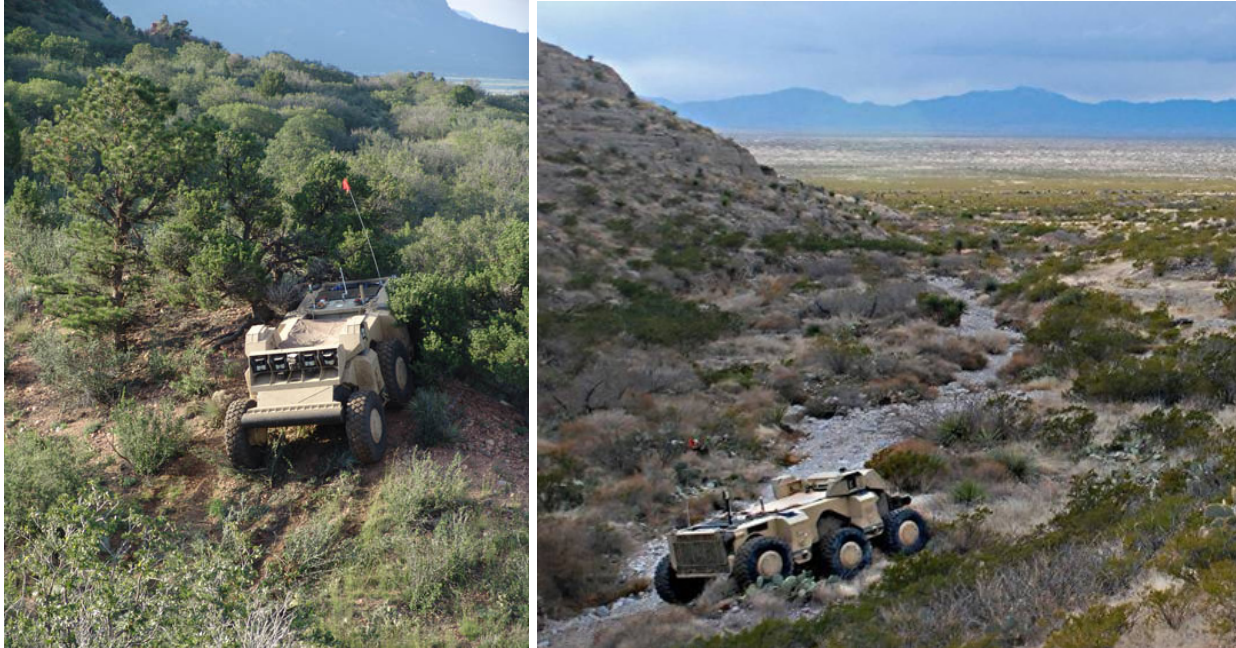
Figure 1: The Crusher autonomous mobility platform is capable of cross-country traverse through rough, complex, and unstructured terrain
