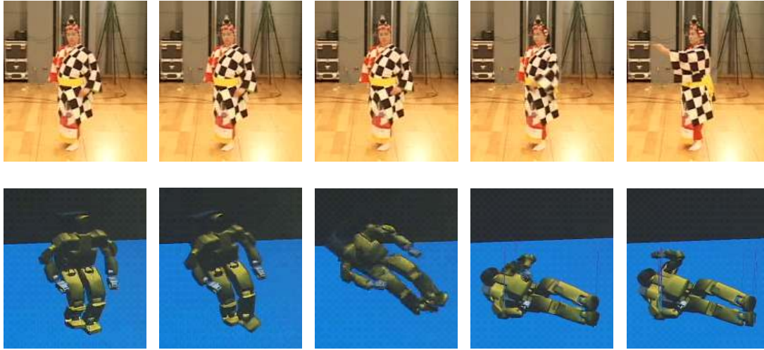
Figure 1.4: An example of falling down. The upper images are the original human motion and the lower images are dynamics simulation of a robot. In this simulation, the robot tried to follow the same motion trajectories as the human. Such an attempt results in the robot immediately falling down like this simulation.
