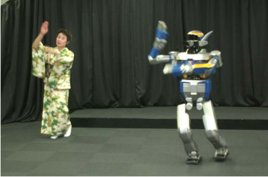
Figure 1.1: The goal of this study. A performance of the robot is reproduced from a human performance. The robot is a biped humanoid robot, and it uses its own legs to support the body during a dance performance.
