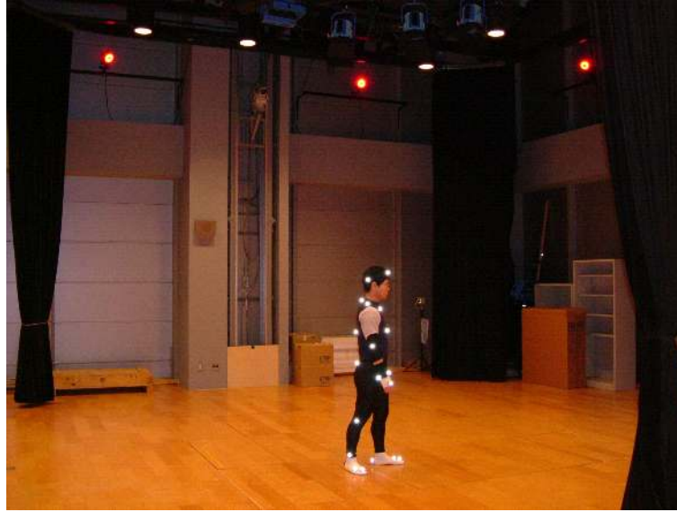
Figure A.1: An optical motion capture system. Around the ceiling, infra-red video cameras are attached. A performer puts on markers, which are illuminated by infra-red lights on the ceiling and shot by the cameras. A performance on the floor is captured by the system.
