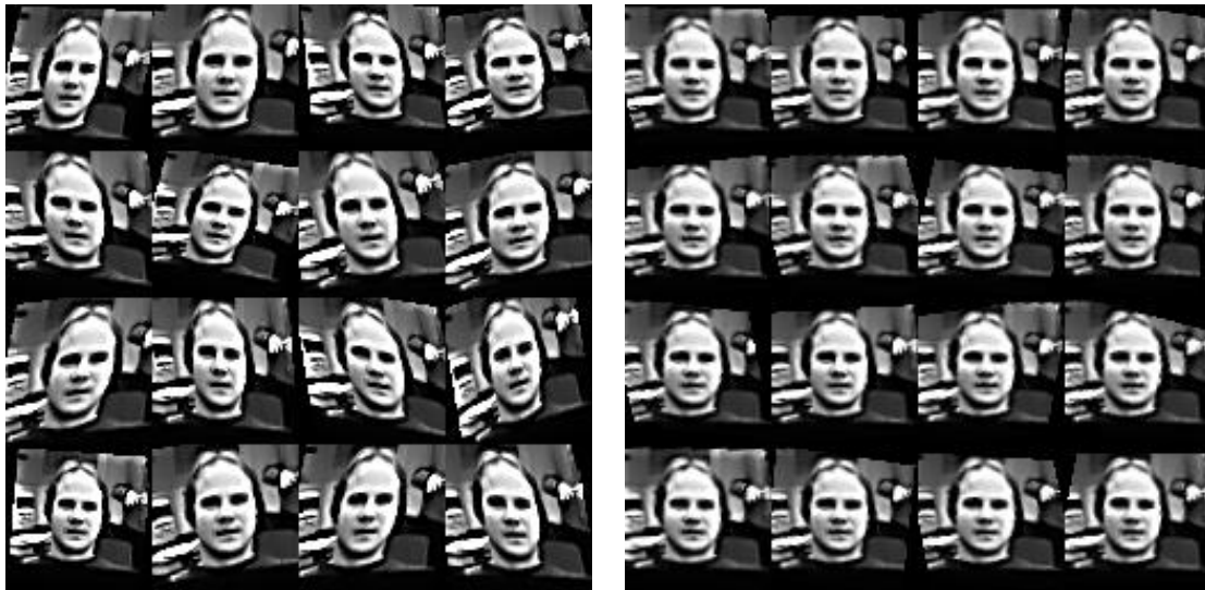
Figure 5-10: Gray scale congealing. On the left are images which have been randomly perturbed in an affine manner. On the right are the congealed versions of the images. The fact that all latent images are the same makes this congealing task artificially easy.
