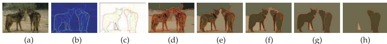
Fig. 10. Overview of our hierarchical segmentation algorithm fPb-OWT-UCM. (a) Test image. (b) Maximal response of contour signals by fPb in (17). (c) Region tree in the UCM. (d)-(h) Segmentations produced by thresholding the UCM in (c) at level 0.01, 0.05, 0.1, 0.3, and 0.5, respectively.
