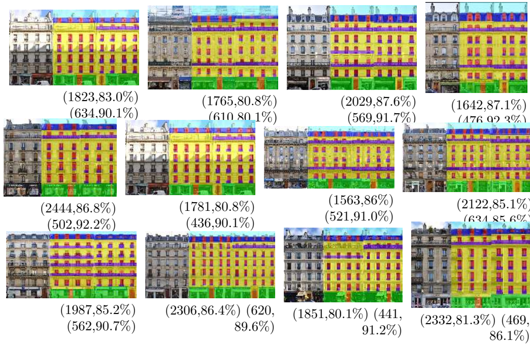
Figure 14: Qualitative results on ECP2011 dataset. Image (left) and segmentation using hand-written grammar (center) and learned grammar \mathcal{G}_{cl} (right) are shown here along with number of episodes for convergence and segmentation accuracy.
