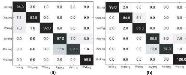
Figure 3. (a) Confusion table for the classification using the optimal number of VWCs ( N_c=177 , average accuracy is 91.31%). (b) Confusion table for the classification using the VWC correlogram. The number of VWC is 60, and 3 quantized distances are used (average accuracy is 94.15%).
