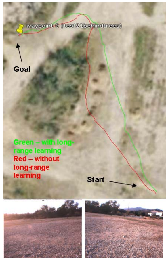
Fig. 6. An overhead map view of the paths taken ( \sim 50\text{m} long) in the Arroyo Seco park with no long-range perception (red) and with long-range learning (green)
