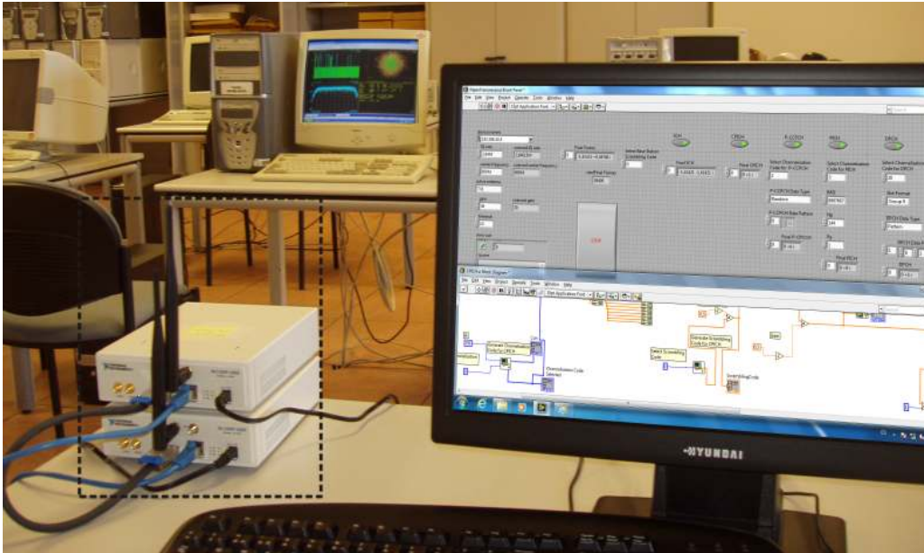
Fig. 1. The developed BTS including the hardware part with NI USRP (dashed box) and software part composed of the computer and the LabVIEW design
