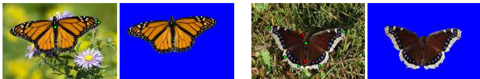
Figure 6: Examples of semi-automatic segmentation: input image (left) and segmentation result (right). Green and red points on the input image indicate the foreground/background points specified by the operator. The operator clicked 2/0 and 6/6 foreground/background points for the left and right images respectively.
