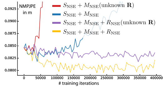
Figure 12. Training error on H36M, with and without estimating the camera rotation \mathbf{R} alongside the human pose \mathbf{p} . Training only converges with the proposed regularization term.
