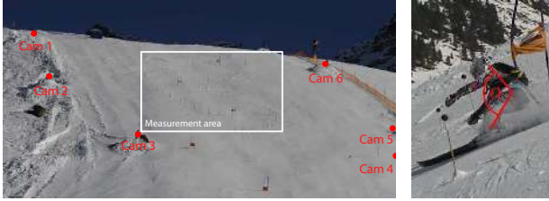
Figure 4. The alpine ski measurement setup. (Left) Six pan-tilt-zoom cameras are placed in a rough circle around the race course. (Right) Metrics such as hip flexion are commonly used for performance analysis.
