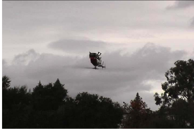
Figure 2.4: Autonomous inverted helicopter flight [Ng et al., 2004b](Picture reprint with permission of Andrew Ng).
