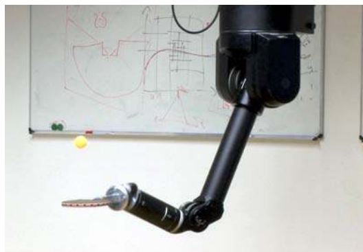
Figure 6.1: This figure illustrates the ball-bouncing task on a Barrett WAM. The goal is to keep the ball bouncing on the racket.
