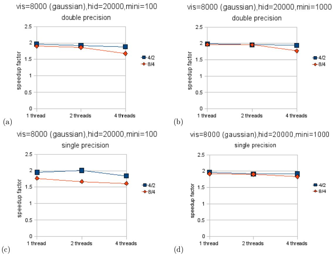
Figure 4.7: This figure shows the speedup factor when parallelizing a Gaussian-to-binary RBM across four machines versus two (blue squares) and eight machines versus four (red diamonds). Notice that doubling the number of machines very nearly doubles the performance.
