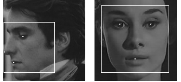
Fig. 3. Feature points and bounding rectangles for two face examples of view around 40^\circ and 90^\circ .
