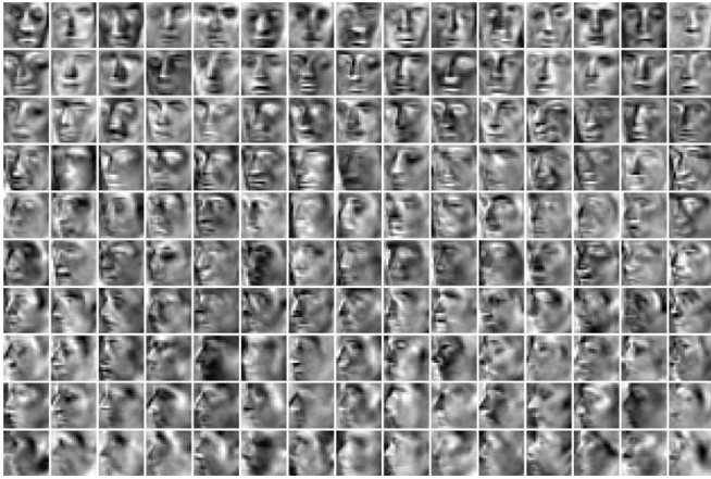
Fig. 10. Basis components learned by using s-ISA. Each row consists of basis components for one view subspace. These components appear more sensible than those learned by u-ISA.
