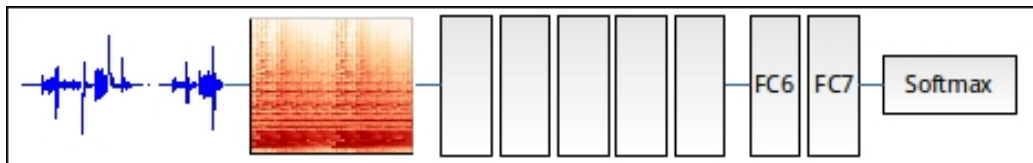
Figure 3: Illustration of the Neural Auditory Embedding method, using a convolutional neural network. The auditory signal is converted to a spectrogram which is fed to the neural network for classification. The pre-softmax layer, FC7, is transferred and taken as the neural audio embedding (NAE) for the given sound file.
