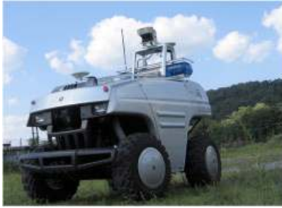
Figure 2. Our test platform is a modified all-terrain vehicle. The panning laser is mounted between the headlights. The fixed laser is mounted on top of the frame in the rear. The vehicle also carries two GPS antennas plus a differential antenna and an inertial measurement unit.
