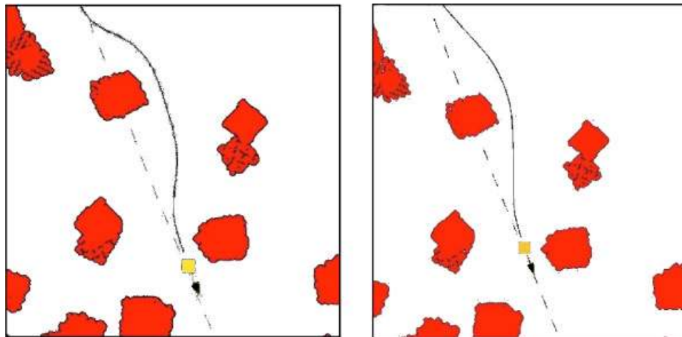
Figure 9. At left, the path driven by the system using the parameters learned from the genetic algorithm. At right, the path driven by the system using the parameters learned by random guessing. They both avoid obstacles, but the genetic algorithm parameters make harder turns.
