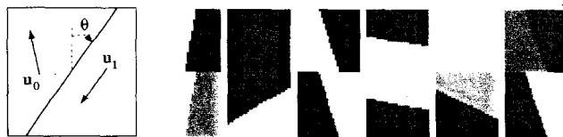
Figure 1: Discontinuity training set. Left: model for generating synthetic flow fields. Right: samples from the training set. The horizontal component is shown above the vertical component. Black denotes pixels moving left or up or u and v respectively. White denotes motion right or down.
