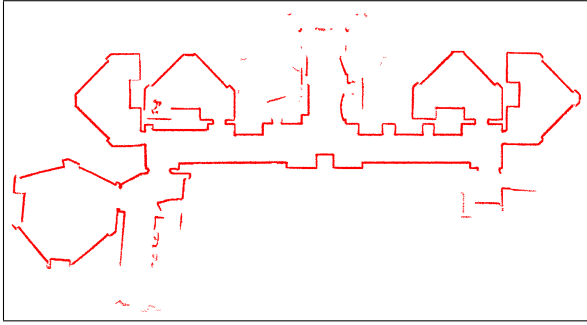
Fig. 6. Scan data and polyline map of the museum in Herakleion. The size of the environment is 38 times 18 m and the input data set contained 268,640 scan points. The resulting polyline map contains 41 polylines with 262 vertices.
