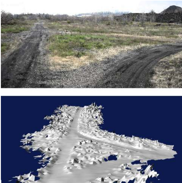
Figure 3: Top: Test area showing dirt roads and vegetation. Bottom: Map of test area using average height.
