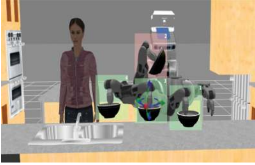
Fig. 4. Interactive feedback. The task here is to move a bowl filled with water. The robot presents a bad trajectory with waypoints 1–2–4 to the user. As feedback user moves waypoint 2 (red) to waypoint 3 (green) using Rviz interactive markers. The interactive markers guide the user to correct the waypoint.
