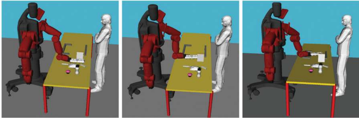
Fig. 14. The learned trajectory for moving an egg carton. Since eggs are fragile the robot moves the carton near the table surface. (Left) Start of the trajectory. (Middle) Intermediate waypoint with egg close to the table surface. (Right) End of the trajectory.
