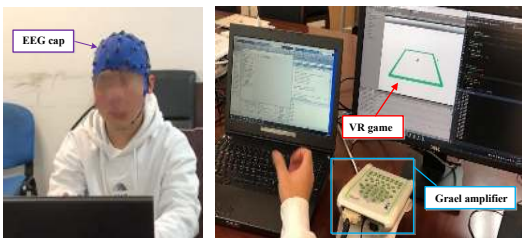
Figure 5: EEG signal recording process and EEG based BCI to control the movement of a virtual ball in 2D space.
