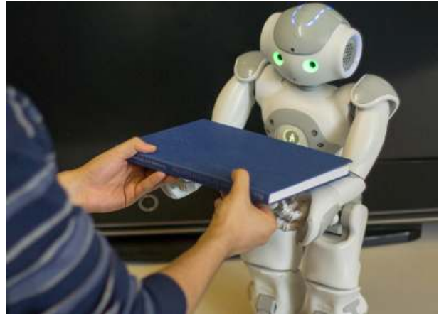
Fig. 1. A humanoid robot receives a book that is handed over by a human interaction partner. The robot learned what to do in this situation by observing a similar situation between two humans.
