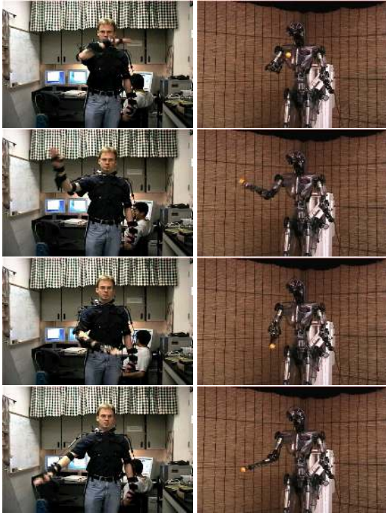
Figure 5: Humanoid robot learning a figure-8 movement from a human demonstration. Left: human demonstration. Right: robot execution. Recording of the robot performance is shown in Figure 6.
