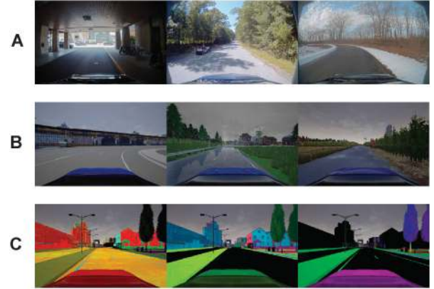
Fig. 3. Training images from various comparison methods: Samples drawn from the real-world, IMIT-AUG (A) and CARLA (B-C). Domain randomization DR-AUG (C) illustrates a single location for comparison.
