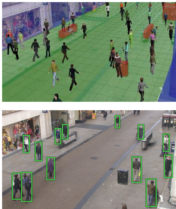
Figure 1. Scene-specific and location-specific pedestrian detection results using geometrically consistent computer generated data.
