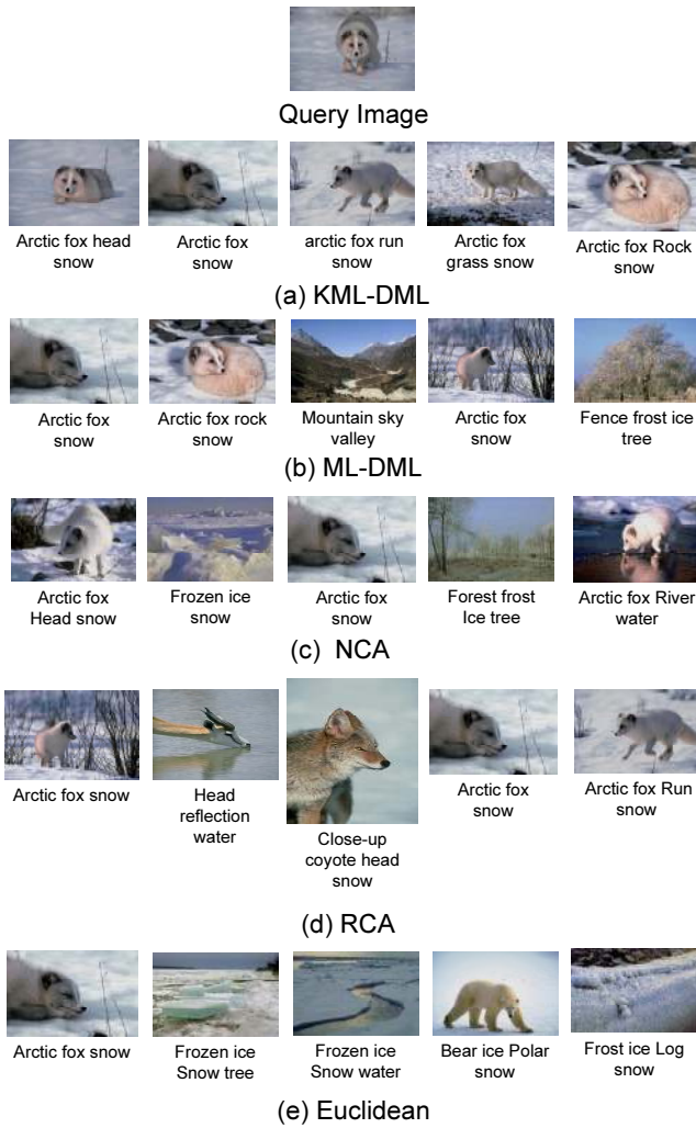
Figure 7: Top 5 retrieved images by KML-DML, ML-DML, NCA, RCA and Euclidean. For each distance metric, the images are ranked by their corresponding distance to the query image. The image with smaller distance is ranked higher.
