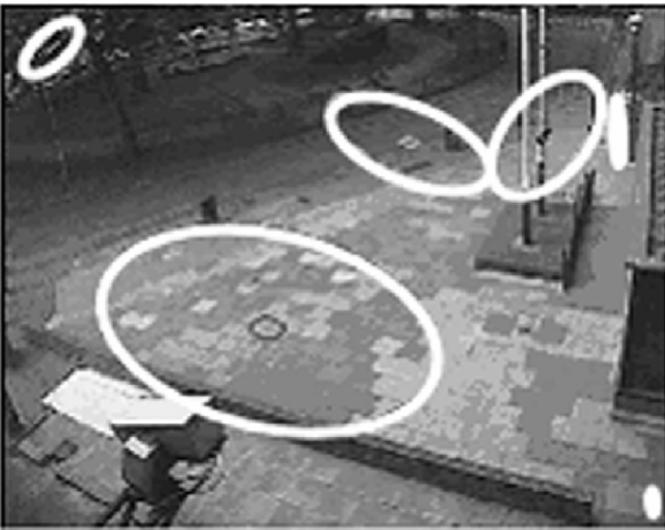
Fig. 6. GMM derived by first run of EM ( N = 6 ). The upper left cluster is caused by the semistationary of the tree branches.
