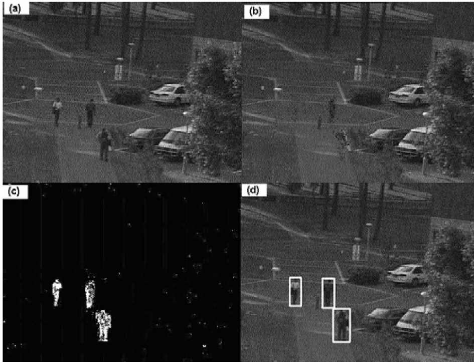
Fig. 1. Motion detection. (a) Original frame. (b) Background model. (c) Foreground pixels. (d) Detected objects.
