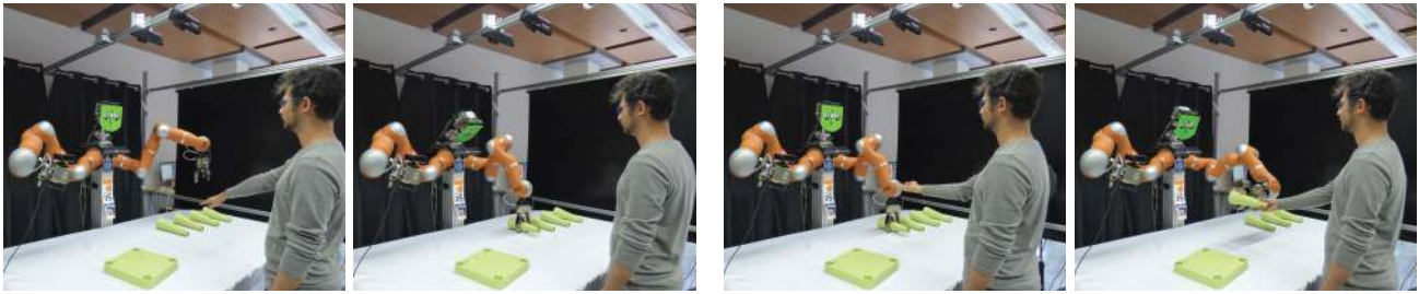
FIGURE 1 | Robin (our robot) assists the user in the assembly of a table. The user performs gestures like pointing and give me to which Robin reacts by grasping the object and handing it over, respectively.
