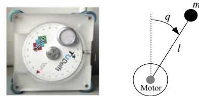
Fig. 10. Inverted pendulum and its schematic.
