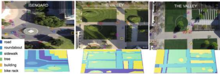
Fig. 2. Some examples of the scenes captured in our dataset. We have annotated all the targets (with bounding boxes) as well as the static scene semantics. The color codes associated to target bounding boxes represents different track IDs.
