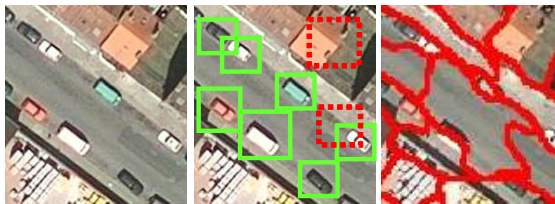
Fig. 1. (Left) An aerial photograph. (Center) Detected cars in the image (solid green = true detections, dashed red = false detections). (Right) Finding “stuff” such as buildings, by classifying regions, shown delineated by red boundaries.
