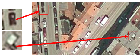
Fig. 2. Example detections from the satellite dataset that demonstrate context. Classifying using local appearance only, we might think that both windows at left are cars. However, when seen in context, the bottom detection is unlikely to be an actual car.
