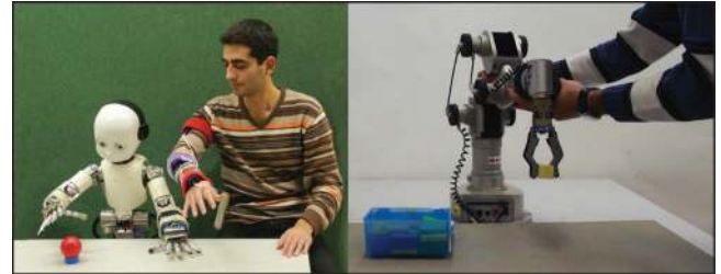
Fig. 1. Demonstrating motions by teleoperating a robot (left) using motion sensors or (right) by back driving it.
