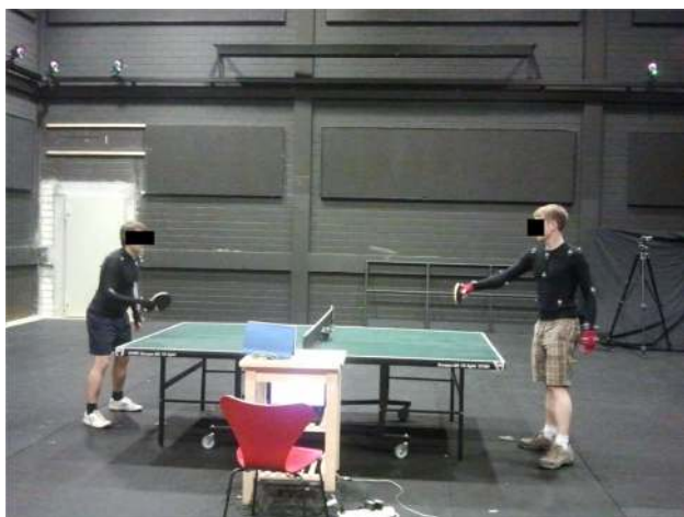
Fig. 6 Experimental setup. A naive player ( right side ) plays against an expert opponent ( left side ). The upper body of both players and the ball are tracked by a motion capture system
