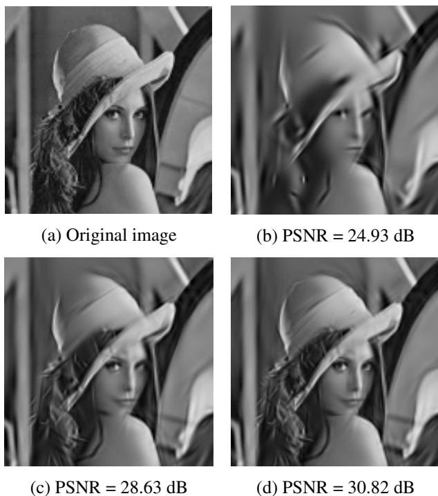
Fig. 2. Lena 128 \times 128 . Original Lena image (a) and its reconstructions using respectively (b) 100, (c) 300 and (d) 500 atoms.
