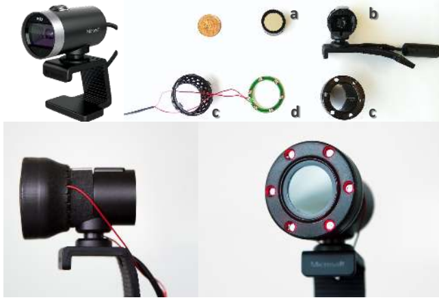
Figure 2: A standard Microsoft LifeCam web camera (top left) is modified to support depth sensing (bottom row). A bandpass filter operating at 850nm (+/-10nm) is added (a), once the front casing is opened and the IR cut filter is removed (b). A new 3D printed case (c) and ring of NIR LEDs (d) are additionally added.
