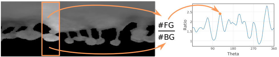
Figure 4: FG/BG ratio: a sliding window moves rightwards to compute the ratio between the number of foreground and background (black) pixels within it. Observe that we have local maxima where leaves are present even when leaves are overlapping.
