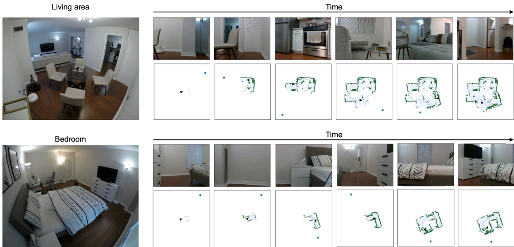
Figure 5: Real-world Transfer. Left: Image showing the living area in an apartment used for the real-world experiments. Right: Sample images seen by the robot and the predicted map. The long-term goal selected by the Global Policy is shown by a blue circle on the map.
