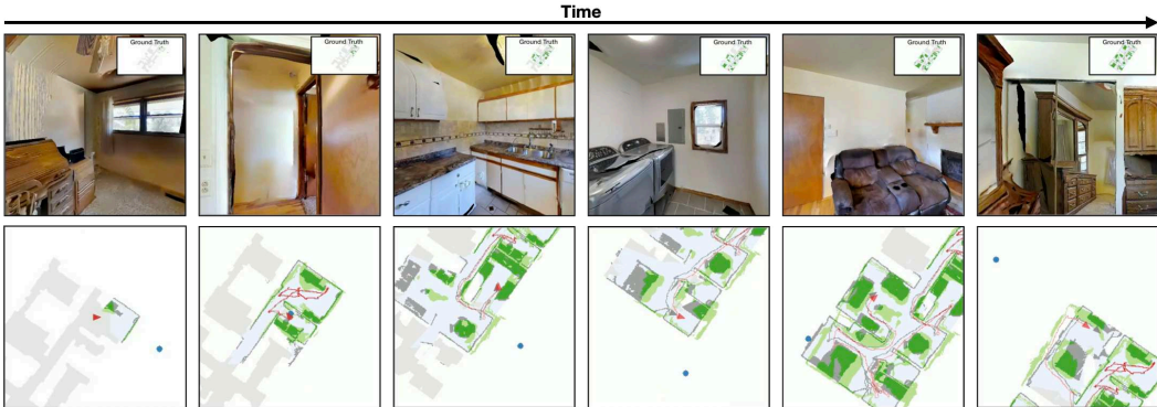
Figure 4: Exploration visualization. Figure showing a sample trajectory of the Active Neural SLAM model in the Exploration task. Top: RGB observations seen by the agent. Inset: Global ground truth map and pose (not visible to the agent). Bottom: Local map and pose predictions. Long-term goals selected by the Global policy are shown by blue circles. The ground-truth map and pose are under-laid in grey. Map prediction is overlaid in green, with dark green denoting correct predictions and light green denoting false positives. Agent pose predictions are shown in red. The light blue shaded region shows the explored area.
