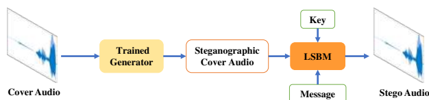
FIGURE 2. The workflow of the ultimate audio steganography model.
