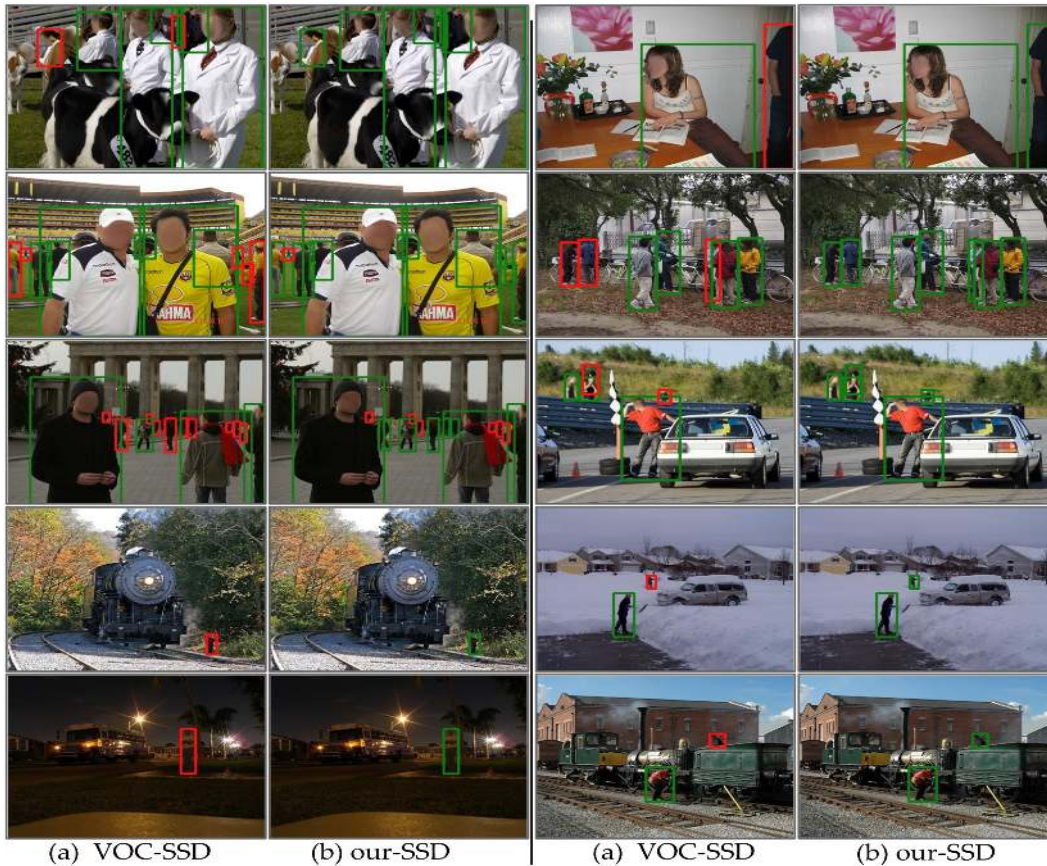
Figure 9: Qualitative results for VOC 2007 test set before and after training SSD with our synthesized data. Green and red boxes show correct and missed detections, respectively. Note that synthetic data helps improve the SSD performance on severely occluded and small instances.
