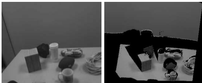
Fig. 2. Image data and depth data captured by our robot. Left: visible light image data. Right: depth data (note: missing back face of objects).
