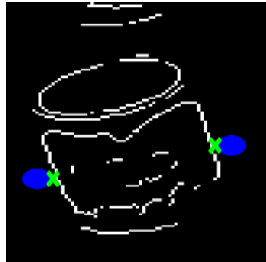
Fig. 3. Edge map (white), contact points (green crosses), and finger placements (blue circles). This edge map is extracted from the mug picture in Figure 1. See text for more details.
