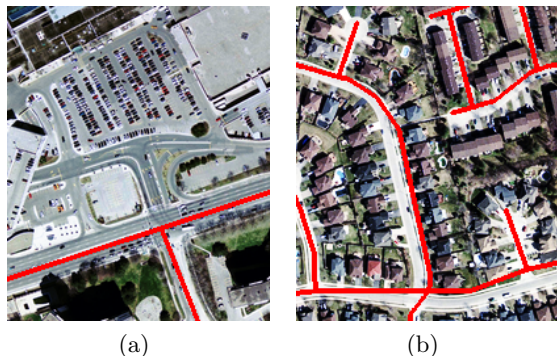
Figure 1. Road locations derived from a map are shown in red. (a) Example of omission noise. (b) Example of registration noise.
