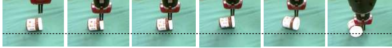
Figure 2: These images depict the robot in the process of displacing the bottle away from the indicated dotted line. In the middle of the poke, the object flips and ends up moving in the wrong direction. Such occurrences are common because the real world objects have complex geometric and material properties. This makes learning manipulation strategies without prior knowledge very challenging.
