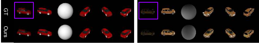
Figure 6: Qualitative examples for 3D shape, texture and light prediction, when exploiting adversarial loss . Purple rectangle : Input image. Left Example : Phong Lighting. Right Example : Spherical Harmonics. First col : Texture and Light. Second col : Texture. Third col : Light. Forth to Sixth col : Texture; different views.
