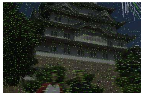
Fig. 3: Green: flow of the estimated epipolar inliers. White: flow of the estimated epipolar outliers. Other features are further computed using these inliers and outliers.
