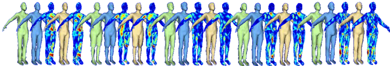
Figure 5. Results from LifeScans in comparison to ground truth shapes (green). We show results computed with ground truth poses (blue) and results of the full method (yellow) with corresponding error heatmaps with respect to ground truth shapes (red means \geq 2 cm).
