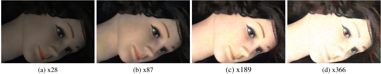
Figure 4. The effect of the amplification factor on a patch from an indoor image in the SID dataset (Sony x100 subset). The amplification factor is provided as an external input to our pipeline, akin to the ISO setting in cameras. Higher amplification factors yield brighter images. This figure shows the output of our pipeline with different amplification factors.
