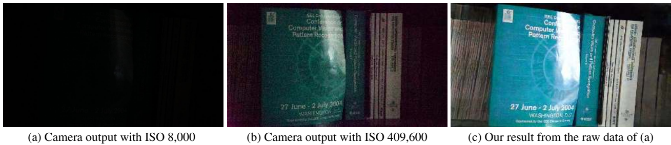
Figure 1. Extreme low-light imaging with a convolutional network. Dark indoor environment. The illuminance at the camera is < 0.1 lux. The Sony \alpha 7S II sensor is exposed for 1/30 second. (a) Image produced by the camera with ISO 8,000. (b) Image produced by the camera with ISO 409,600. The image suffers from noise and color bias. (c) Image produced by our convolutional network applied to the raw sensor data from (a).
