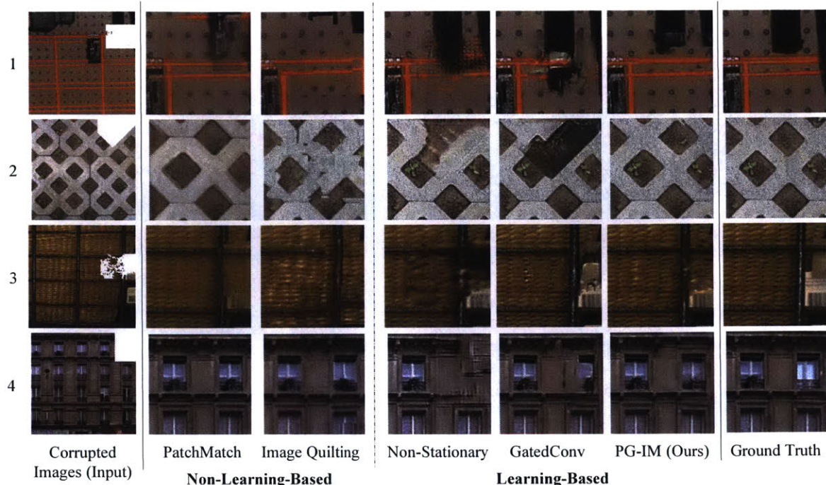
Figure 10-6: Corrupted input images and inpainting results (zoomed-in) by PG-IM and the baselines. The white pixels in the leftmost column are missing pixels to inpaint. The rightmost column shows the ground-truth patches. PG-IM inpaints realistic image patches that are consistent with the intricate global regularity and meanwhile different from the original, ground-truth patches.
