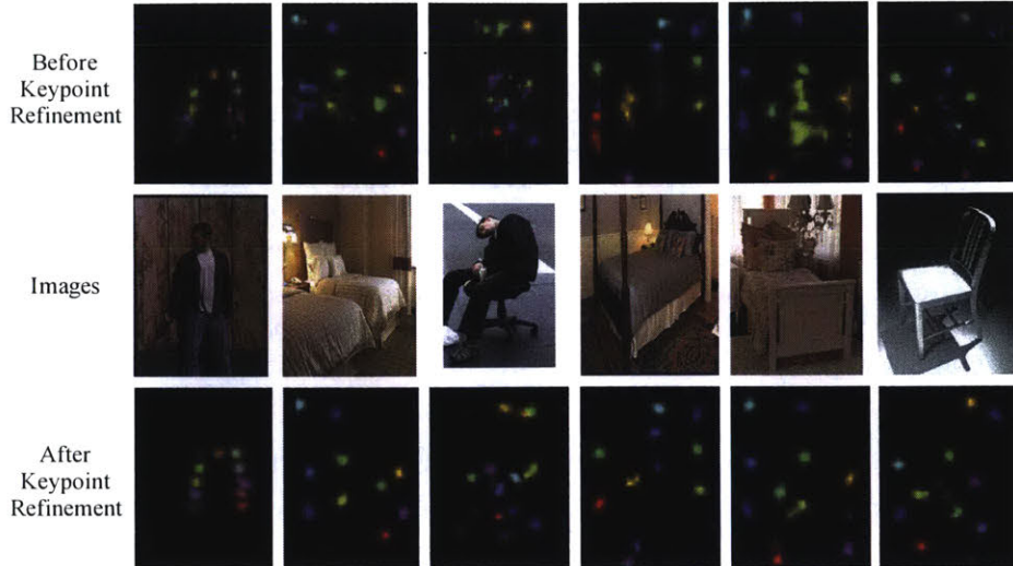
Figure 2-6: Qualitative results on 2D keypoint estimation from a single image, where each color corresponds to a keypoint. The keypoint refinement step cleans up false positives and produces more regulated predictions.
